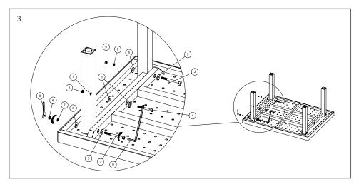
3. Attach all bolts, nuts and discs loosely. Once they are in place, tighten.
